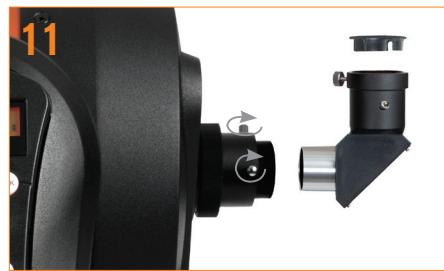
11 Remove the cap on the rear of the telescope. Insert the silver barrel of the star diagonal into the visual back. Tighten the silver set screw to secure.
