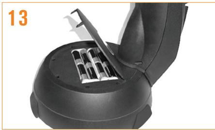
13 Remove the battery cover from the center of the base by gently lifting on the round portion of the cover. Insert 8 AA batteries into the holder and reattach the battery cover. Be careful to insert the batteries in the correct polarity.
