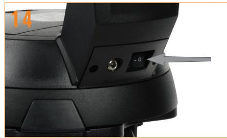
14 Turn on the power switch located at the base of the fork arm.
