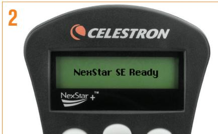
The display reads "NexStar SE Ready." Press ENTER to begin the alignment procedure.
