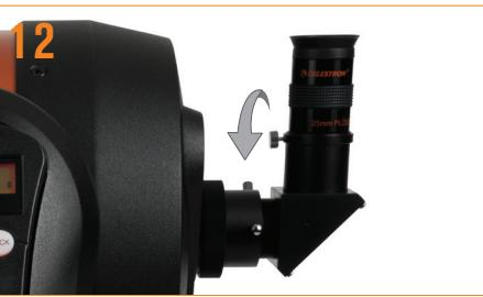
12 Insert the silver barrel of the 25mm eyepiece into the star diagonal. Tighten the silver screw to secure.
