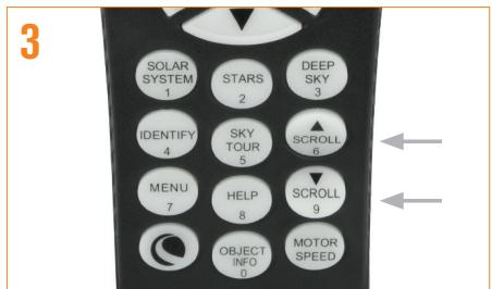
Use the SCROLL UP and SCROLL DOWN buttons (located on #6 and #9 keys respectively) to select "SkyAlign" then press ENTER.
