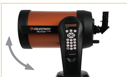
17 With the telescope powered on, use the hand control directional slew buttons (the arrow keys) to move the scope up, down, left, or right. The altitude axis (up & down) also has a slip clutch that you can move by hand at any time. The azimuth axis (left and right) does not. Forcing the scope left and right without using the hand control can result in damage to the gears.
