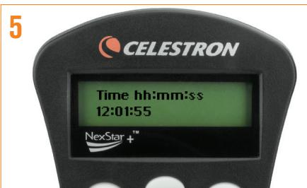
Use the numeric keypad enter the current time. Press ENTER to continue. Press UNDO to backspace. If you entered the time in 12-hour format, you will need to select AM or PM.
