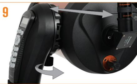
9 To adjust the balance or remove the tube from the base, simply loosen the quick-release clamp knob and slide the tube back towards the rear cell of the tube. Hold the tube firmly when mounting or dismounting. Ensure the dovetail clamp is tight before releasing the tube.
